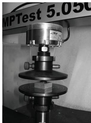
Figure 1. Measurement Compression set.
