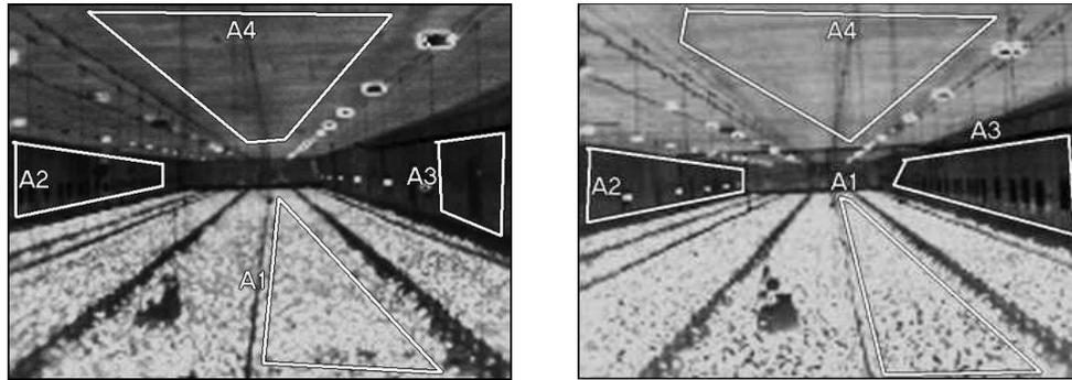
**Figure 4.** The thermograms of the surface areas inside the poultry house 1 (left) and 2 (right). Where A1 is the evaluated surface area of the chickens on the floor; A2 is the south wall; A3 is the north wall; A4 is the ceiling.
