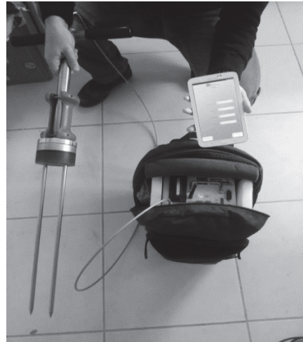
Figure 1. TDR–slammer with a 40 cm waveguide.
