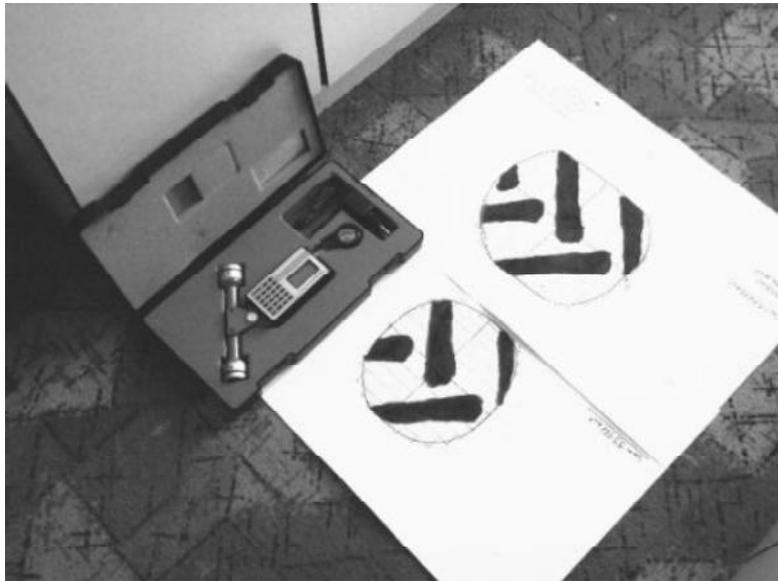
**Figure 2.** Koizumi KP-90N digital polar planimeter.
