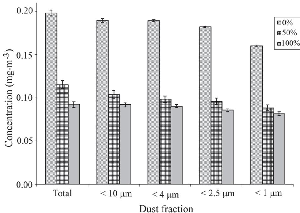
**Figure 4.** The total concentration and size of dust particles in the laboratory of adhesive bonding.
