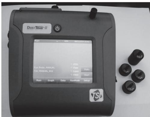
**Figure 1.** The DustTrak™ II Aerosol Monitor 8530.
