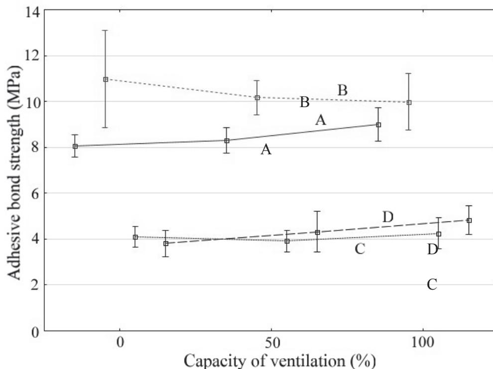
**Figure 3.** Influence of capacity of ventilation in hall determined for adhesive bonding on adhesive bond strength.
