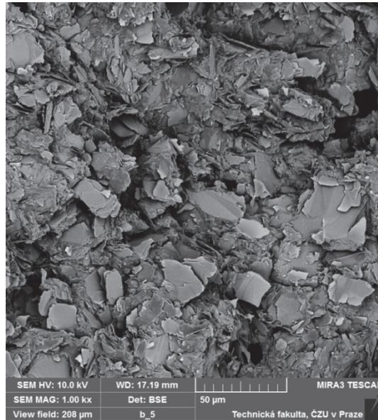
**Figure 5.** SEM images of fracture surface of sample – Back-scattered electrons (BSE).
