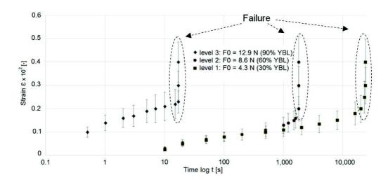
Figure 4. Measured creep curves of Ensete fibres.
