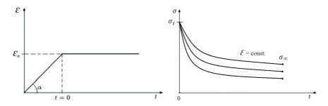
Figure 2. Typical loading history (left) and measured curves (right) in a stress relaxation test.
