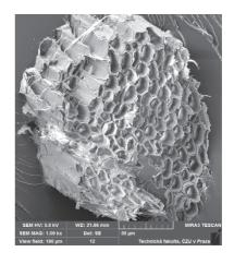
Figure 3. SEM image of Ensete fibre.
