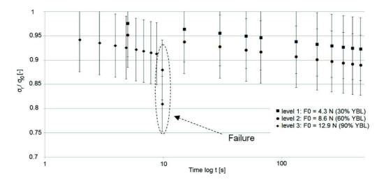
Figure 5. Measured stress relaxation curves of Ensete fibres.
