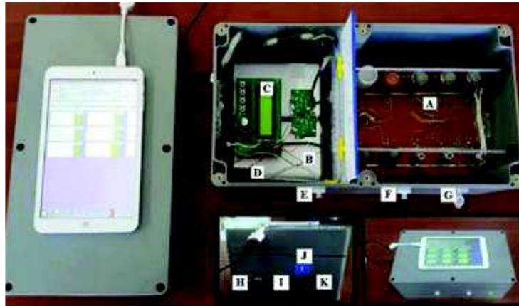
**Figure 2.** Modified e-nose system [A: sensor array, B: power bank, C: micro pump control unit, D: micro pump, E: sample air inlet, F: sample air outlet (reference gas inlet if needed), G: reference gas outlet (if needed), H: USB 4 port to tablet PC, I: sensor array power switch and USB charging port, J: power indicator LEDs, and K: micro pump power switch and USB charging port].
