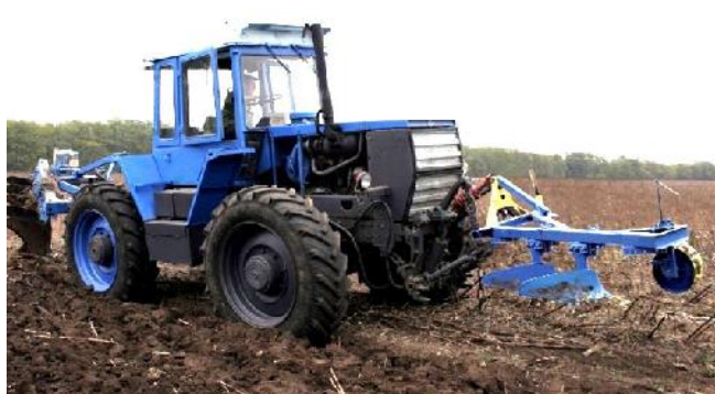
Figure 1. Tractor-implement unit operating on the 'push-pull' principle.
