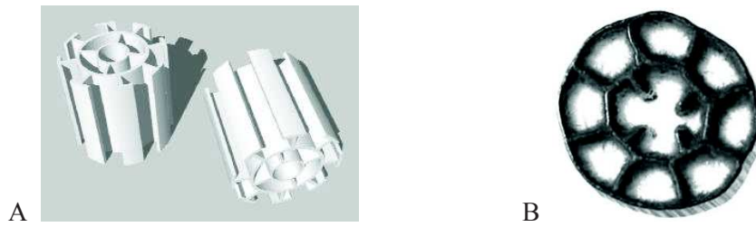
Figure 1. Schematic illustration of a plastic carrier (A) and particular of biofilm (B).
