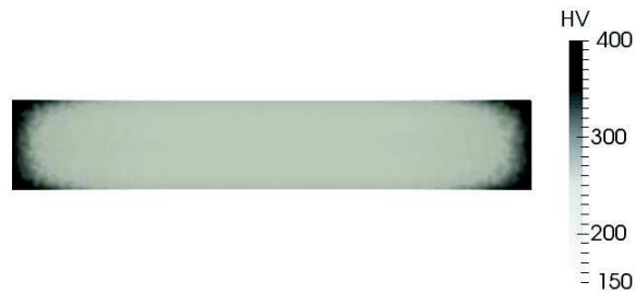
Figure 3. Hardness in cross section (near the hole in Fig. 4) of chisel after heat treatment.
