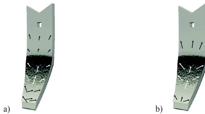
Figure 4. Vectors of force (a) and velocity (b) from DEM.
