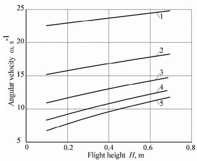
**Figure 4.** Relation between spiral's angular velocity  $\omega$  and potato tuber's flight height  $H$  at various values of tuber's radius  $R_b$ : 1)  $R_b = 0.035$  m; 2)  $R_b = 0.040$  m; 3)  $R_b = 0.045$  m; 4)  $R_b = 0.050$  m; 5)  $R_b = 0.055$  m.
