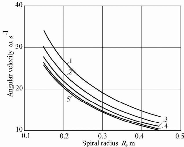
**Figure 2.** Relation between spiral's angular velocity  $\omega$  and spiral's radius  $R$  at various values of angle  $\chi$ : 1)  $\chi = 25^\circ$ ; 2)  $\chi = 35^\circ$ ; 3)  $\chi = 45^\circ$ ; 4)  $\chi = 55^\circ$ ; 5)  $\chi = 65^\circ$ .
