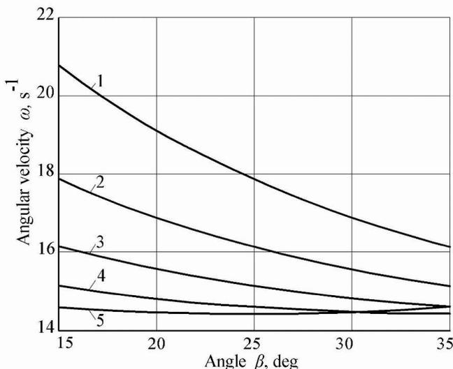
**Figure 5.** Relation between spiral's angular velocity  $\omega$  and conveyor's tilt angle  $\beta$  at various values of angle  $\chi$ : 1)  $\chi = 25^\circ$ ; 2)  $\chi = 35^\circ$ ; 3)  $\chi = 45^\circ$ ; 4)  $\chi = 55^\circ$ ; 5)  $\chi = 65^\circ$ .
