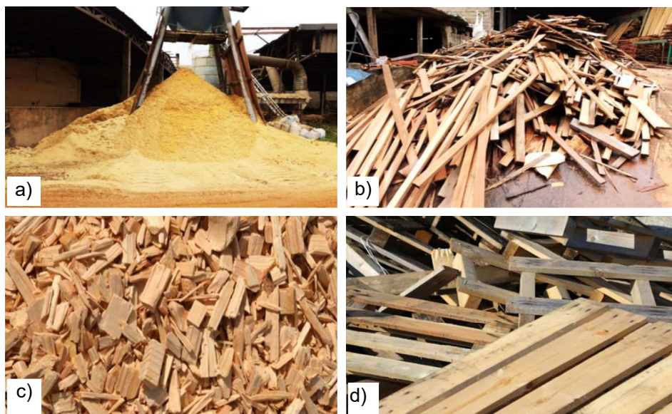
Figure 1. Different forms of wood waste biomass: a) pile of sawdust; b) wooden offcuts or scraps from lumber; c) wood chips; d) old pallets.
