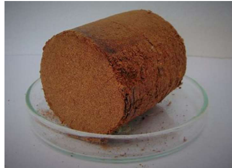
Figure 5. Produced bio-briquette sample before experimental testing.
