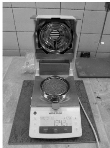
**Figure 5.** HE43 moisture analyser by Mettler-Toledo.
