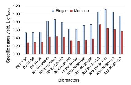
Figure 3. Specific biogas and methane yield from bioreactors with wheat straw pellets or its cofermentation with molasses, sunflower oil and catalyst Metaferm.
