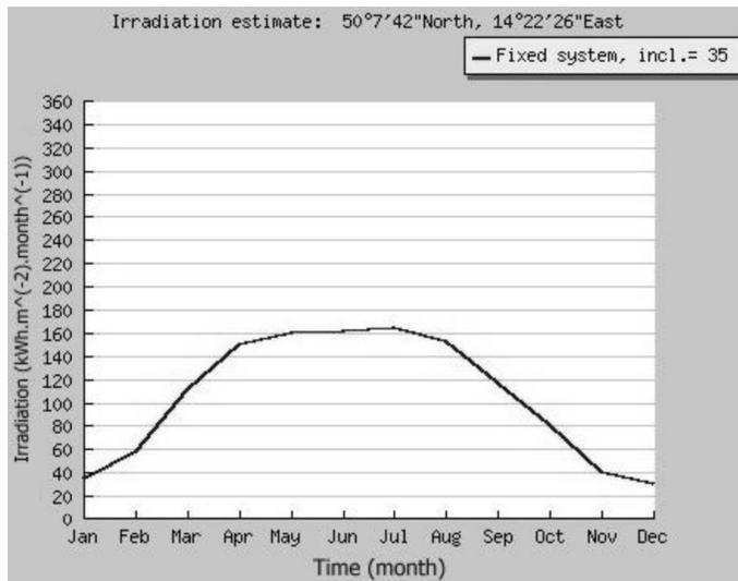
**Figure 4.** Irradiation estimate for Prague.
