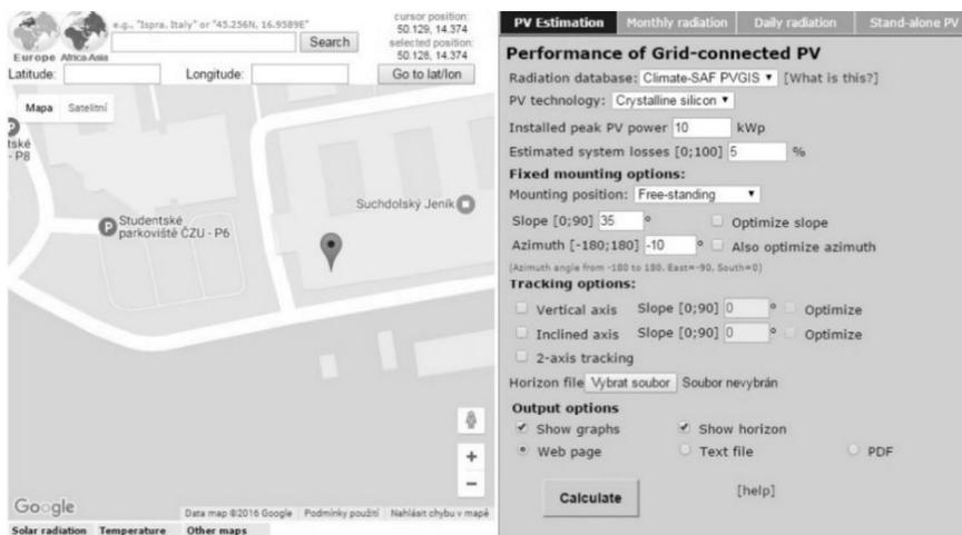
**Figure 2.** GUI of PVGIS with parameters for PV installation in Prague.
