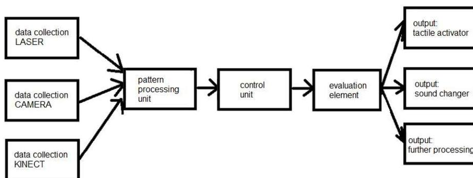
**Figure 1.** Block diagram of the tactile navigation system.
