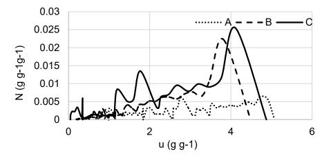
**Figure 5.** Drying rate N (g  $g^{-1}$ min<sup>-1</sup>) of 3 alfalfa samples as a function of water content u (g  $g^{-1}$ ) during the drying process.
