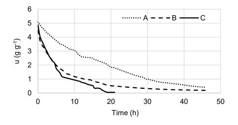
Figure 1. Water content, dry basis u (g g<sup>-1</sup>) of all 3 alfalfa samples during the drying process.
