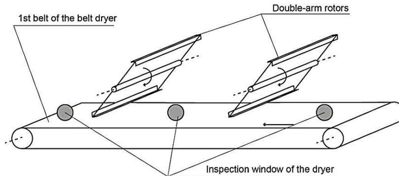
**Figure 1.** Scheme of placing of two double-arm rotors above the first belt of belt dryer (rotor diameter – 840 mm, rotor rotational frequency –  $2.5\text{--}3\text{ min}^{-1}$ ).
