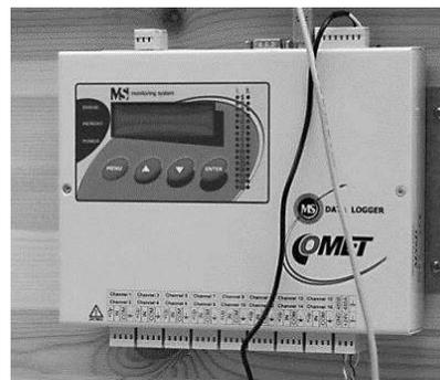
**Figure 6.** Comet MS6D multi-channel data logger.
