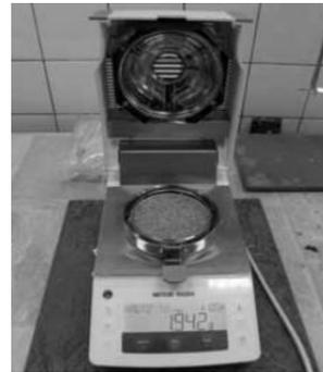
**Figure 8.** Mettler-Toledo HE43 moisture analyser.
