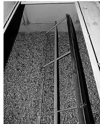
**Figure 2.** Rotor installed above the first belt of belt dryer.
