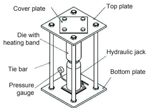
**Figure 1.** The developed experimental biomass briquetting Press.
