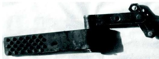
**Figure 7.** Cleaning element that can hold flexible blades of different lengths and with different elastic moduli (manufactured from different materials: rubber, plastic, cord-reinforced rubber, belts).
