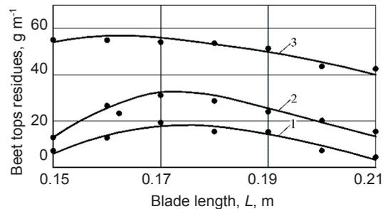
**Figure 8.** Relation between amount of haulm residues on sugar beet root crowns after their cleaning and cleaning blade length  $L$  at different angular velocities of rotation of cleaner's drive shaft: 1– $734 \text{ rad s}^{-1}$ ; 2– $540 \text{ rad s}^{-1}$ ; 3– $448 \text{ rad s}^{-1}$ .
