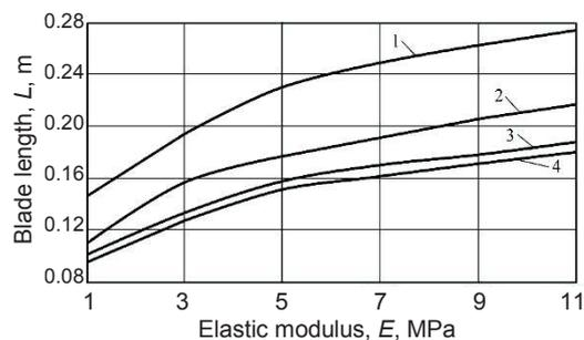
**Figure 6.** Dependence of length  $L$  of the cleaning blade upon its modulus of elasticity  $E$ : 1)  $\varphi_1 = 60^\circ$ ; 2)  $\varphi_1 = 70^\circ$ ; 3)  $\varphi_1 = 80^\circ$ ; 4)  $\varphi_1 = 90^\circ$ .
