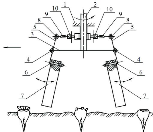
**Figure 1.** A design and technological scheme of the new cleaner of the root crop heads without extraction from the ground, with a vertical drive shaft (Bulgakov et al., 2018): 1 – the frame; 2 – the vertical drive shaft; 3 – the disk; 4 – the spherical joints of the disk; 5 – the double-arm levers; 6 – the axes; 7 – the flexible cleaning blades; 8 – the spherical joints of the levers; 9 – the pairs of screws; 10 – the kinematic mechanisms.
