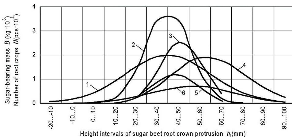
**Figure 7.** Distribution of heights of sugar beet root crown protrusion above soil surface where  $m = 40$  mm:  $N$  – number of roots: 1)  $\sigma = 10$  mm; 2)  $\sigma = 20$  mm;  $B_z$  – sugar-bearing mass above ground: 3)  $\sigma = 10$  mm; 4)  $\sigma = 20$  mm;  $B_{3n}$  – sugar-bearing mass above ground containing haulm: 5)  $\sigma = 10$  mm; 6)  $\sigma = 20$  mm.
