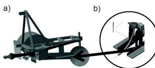
**Figure 1.** Laboratory unit (3D model) for measurement of height that sugar beet roots protrude above the soil level (a) and layout of its measuring unit (b).
