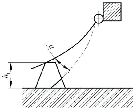
**Figure 5.** Schematic model of measuring root crown protrusion.
