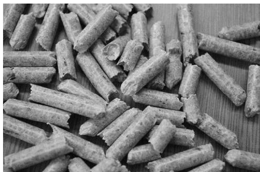
Figure 1. Pellets made from the residual processing spruce wood.
