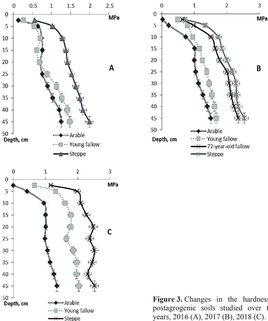
**Figure 3.** Changes in the hardness of postagrogenic soils studied over three years, 2016 (A), 2017 (B), 2018 (C).
