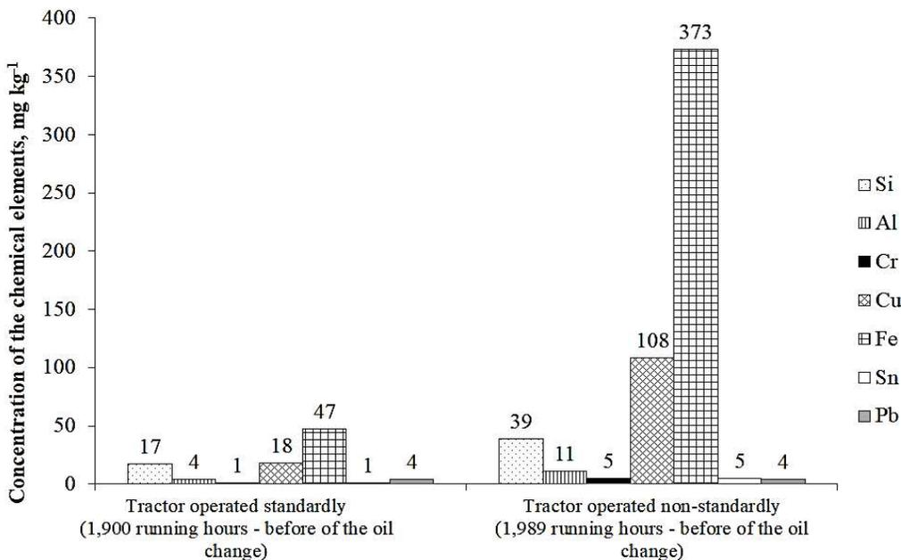
**Figure 2.** The oil contamination of the tractors operated standardly and non-standardly.
