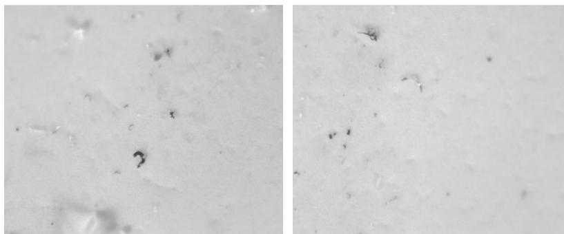
**Figure 4.** The filter patch of the oil Shell Donax 5W30 from the tractor operated standarily.
