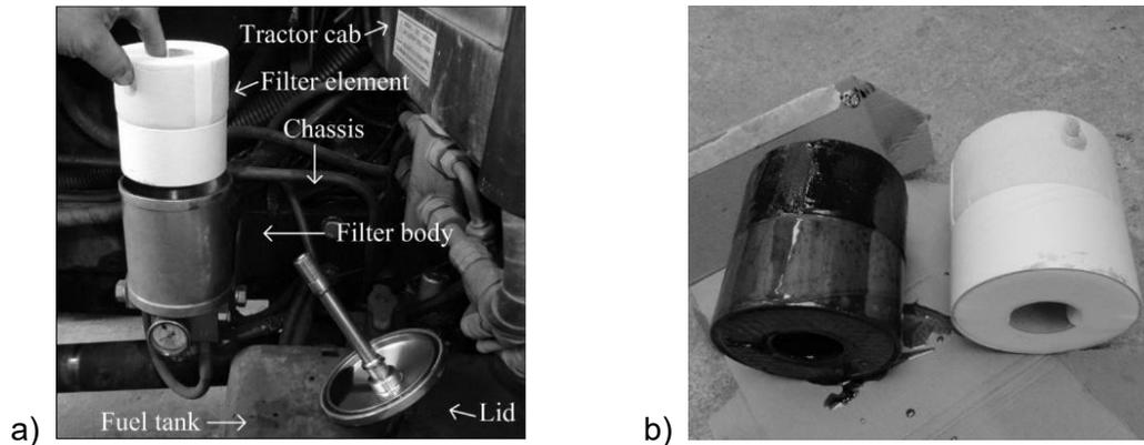
**Figure 8.** The change of the filter element after the tractor testing operation with the by-pass filtration system: a) placement of the filter body in the cab-behind-engine; b) the new and the used filter element.
