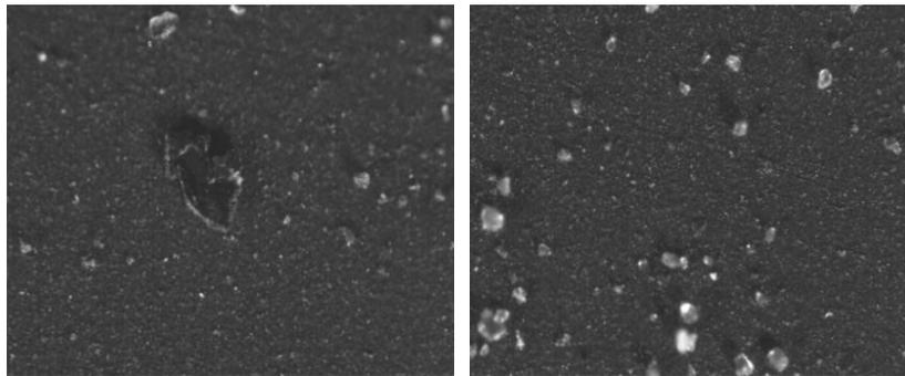
**Figure 3.** The filter patch of the oil PP 90 from the tractor operated non-standarily.
