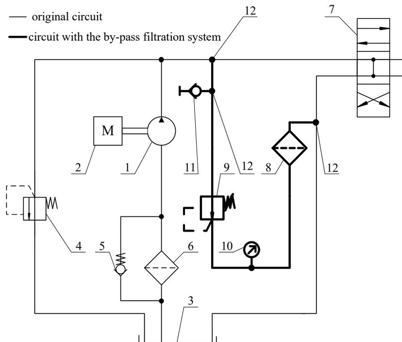
**Figure 7.** Tractor hydraulic circuit with the by-pass filtration system: 1 – hydraulic pump; 2 – combustion engine; 3 – oil fill of the tractor transmission; 4 – pressure relief valve; 5 – one direction valve; 6 – operational filter; 7 – directional control valve; 8 – by-pass filter; 9 – pressure-reducing valve; 10 – pressure gauge; 11 – minimess type valve; 12 – T-fitting.
