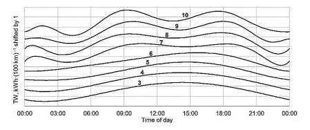
**Figure 7.** Polynomial regression lines with equalised endpoints for traction work per 100 km for polynomial orders from 3 to 10 in the direction against the green wave.
