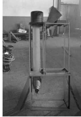
Figure 12. General view of experimental unit for research into vibration and aspiration separation of sunflower seeds.
