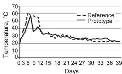
Figure 9. Composting Temperature vs Time.
