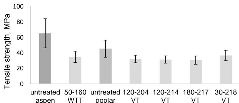
**Figure 2.** The tensile strength of veneer samples.
