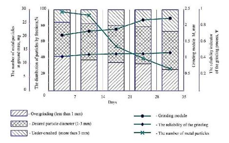
Figure 1. Experimentally determined indicators of grinding crushers DM-10.
