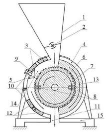
**Figure 2.** Scheme of a prototype rotary crusher: 1 – receiving hopper; 2 – damper; 3 – plugs in add. places of a loading window; 4 – a stator; 5 – cutting element; 6 – a rotor; 7 – a removable surface of a rotor; 8 – fastenings of a surface of a rotor; 9 – a lining for variation of a backlash; 10 – fastening and caps in add. locations of the counter-blade; 11 – discharge hopper; 12 – plugs in add. places of unloading; 13 – limiting lip; 14 – crushing chamber; 15 – frame.
