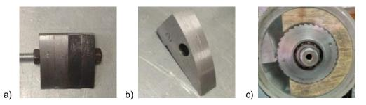
**Figure 3.** General view of: the cutting element (a), markings its segments (b) and the grinding zone in a horizontal rotary crusher (c).
