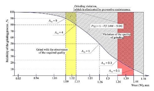
Figure 5. Dependence of reliability grinding process of grain materials wear riffles cutting element.
