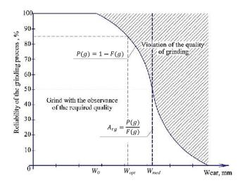
**Figure 4.** Theoretical probability of failure-free operation of the rotor crusher depending on the wear of the rotor and stator.
