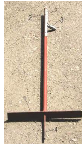
Figure 5. Instrument for measuring tillage depth: 1 – cross bar; 2 – measuring scale; 3 – lever; 4 – rod.
