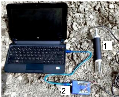
Figure 3. Soil moisture content measuring kit: 1 – SHS-1; 2 – Arduino Uno.
