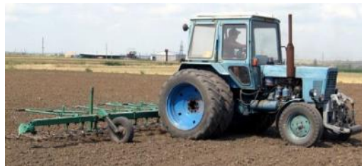
Figure 2. Combined tractor and harrow unit during fallow field tillage.
