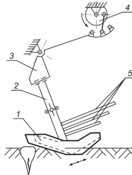
**Figure 2.** Design and process schematic model of vibrational lifting tool: 1 – lifting shares; 2 – posts; 3 – share spacing adjustment system; 4 – vibration drive with share oscillation amplitude and frequency adjustment system; 5 – guide pins.
