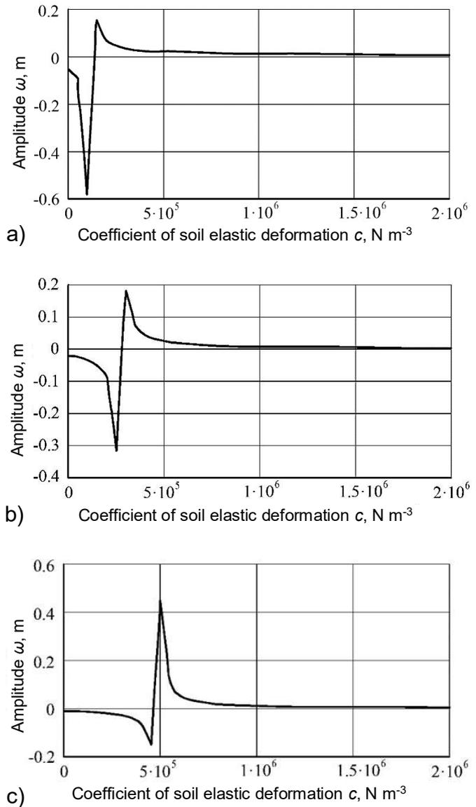
**Figure 4.** Relation between amplitude of forced transverse root body oscillations on one hand and coefficient of elastic soil deformation  $c$  and perturbing force frequency  $\nu$  on the other hand for root's cross-section at point of its gripping ( $z = z_1 = 0.15 \text{ m}$ ): a)  $\nu = 10 \text{ Hz}$ ; b)  $\nu = 15 \text{ Hz}$ ; c)  $\nu = 20 \text{ Hz}$  (perturbing force amplitude  $H = 500 \text{ N}$ ,  $b = 6.5 \text{ N s}^2 \text{ m}^{-3}$ ,  $c = 0-20 \text{ N m}^{-3}$ ).
