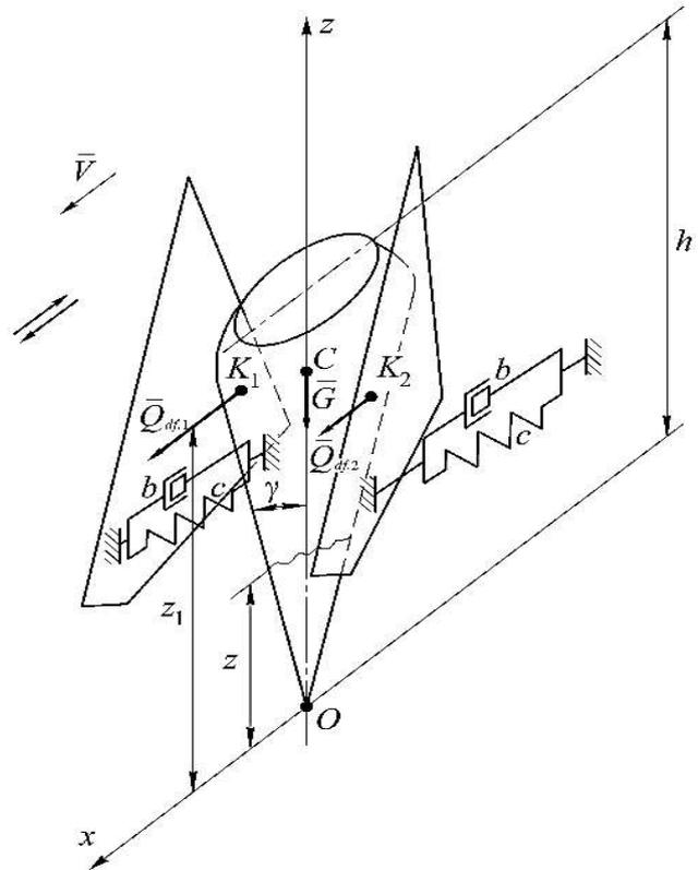
**Figure 3.** Equivalent schematic model of transverse oscillations performed by root sitting in soil during its vibrational lifting.
