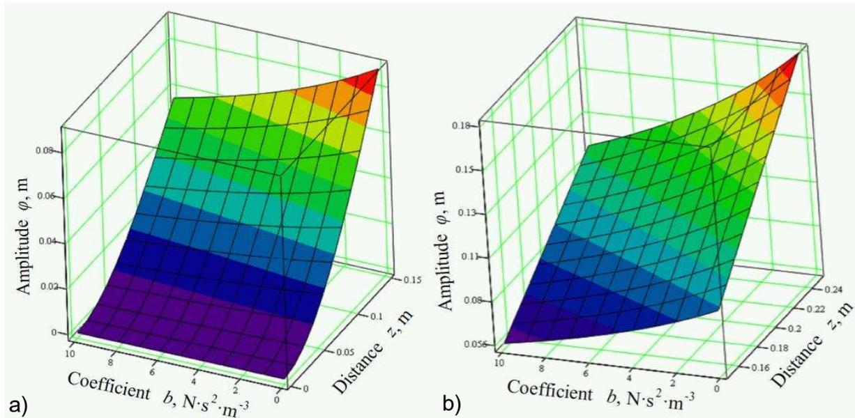
**Figure 7.** Relation between amplitude of forced transverse root body oscillations on one hand and soil damping coefficient  $b$  and distance from root's cross-section to conventional point of its fixing  $z$  on the other hand: a)  $z = 0-0.15$  m; b)  $z = 0.15-0.25$  m; (perturbing force amplitude  $H = 500$  N, perturbing force frequency  $\nu = 10$  Hz).
