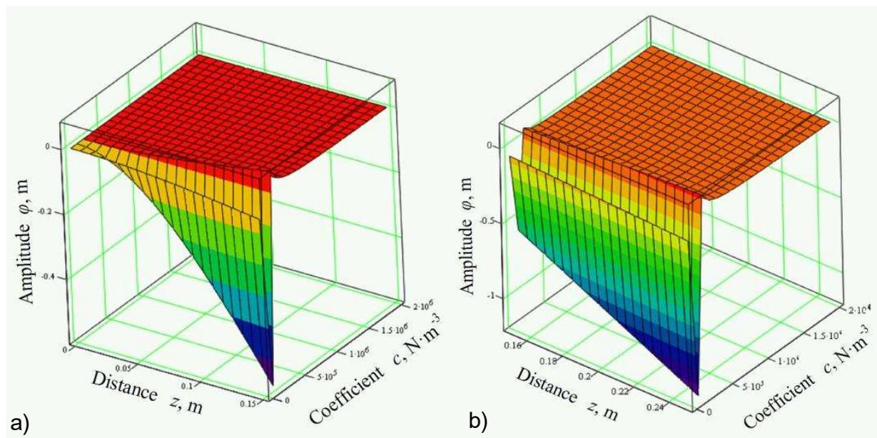
**Figure 5.** Relation between amplitude of forced transverse root body oscillations on one hand and coefficient of elastic soil deformation  $c$  and distance from root's cross-section to conventional point of its fixing  $z$  on the other hand: a)  $z = 0\text{--}0.15$  m; b)  $z = 0.15\text{--}0.25$  m; (perturbing force amplitude  $H = 500$  N,  $b = 6.5$  N s<sup>2</sup> m<sup>-3</sup>, perturbing force frequency  $\nu = 10$  Hz).
