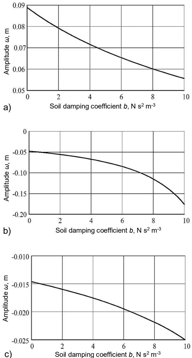
**Figure 6.** Relation between amplitude of forced transverse root body oscillations on one hand and soil damping coefficient  $b$  and perturbing force frequency  $\nu$  on the other hand for root's cross-section at point of its gripping by tool ( $z = z_1 = 0.15$  m): a)  $\nu = 10$  Hz; b)  $\nu = 15$  Hz; c)  $\nu = 20$  Hz (perturbing force amplitude  $H = 500$  N,  $b = 0-10 \text{ N s}^2 \text{ m}^{-3}$ ,  $c = 2 \cdot 10^5 \text{ N m}^3$ ).
