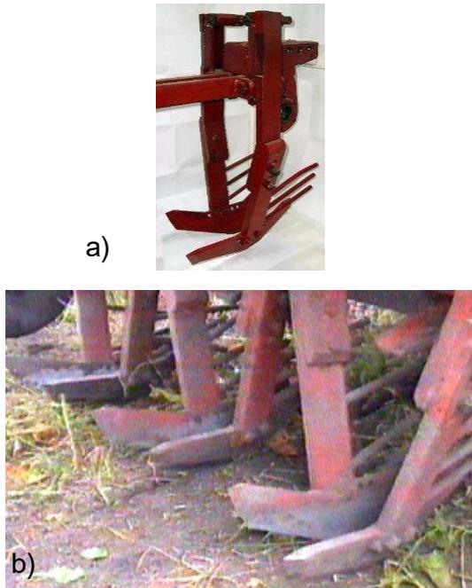
**Figure 1.** Vibrational lifting tool: a – general appearance; b – tools installed on experimental multiple-row root harvester.
