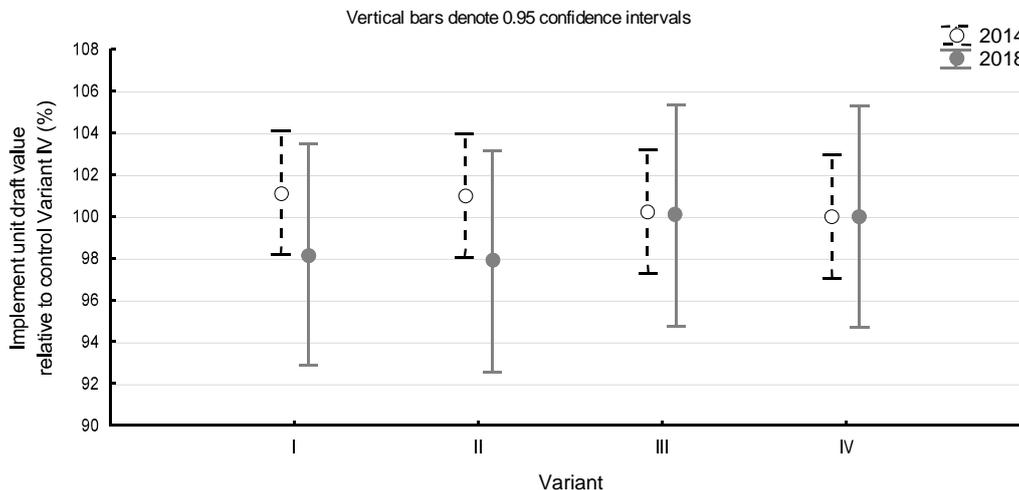
**Figure 2.** Graph comparing relative differences of implement unit draft values for individual variants in autumn 2014 and 2018 (Variants: I – FYM with Z’ fix; II – FYM with Z’ fix + NeoSol; III – FYM; IV – Control as 100%).
