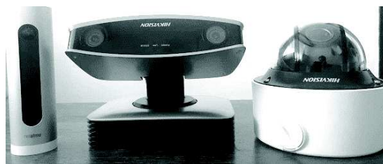
Figure 1. Tested recognition camera system (from the left: Netatmo Welcome, HIKVISION iDS-2CD8426G0/F-I, HIKVISION DS-2CD4D36FWD-IZS).
