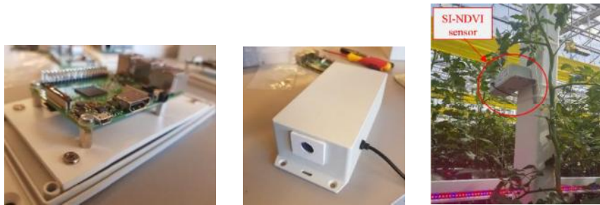
Figure 2. SI-NDVI sensor prototype and placement in the greenhouse.
