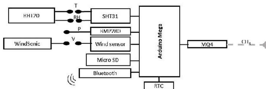
**Figure 1.** Sketch of the measured variables setup: stand-alone sensors. Measured variables: temperature (T), relative humidity (RH), air velocity (V) and atmospheric pressure (P) and methane (CH<sub>4</sub>).
