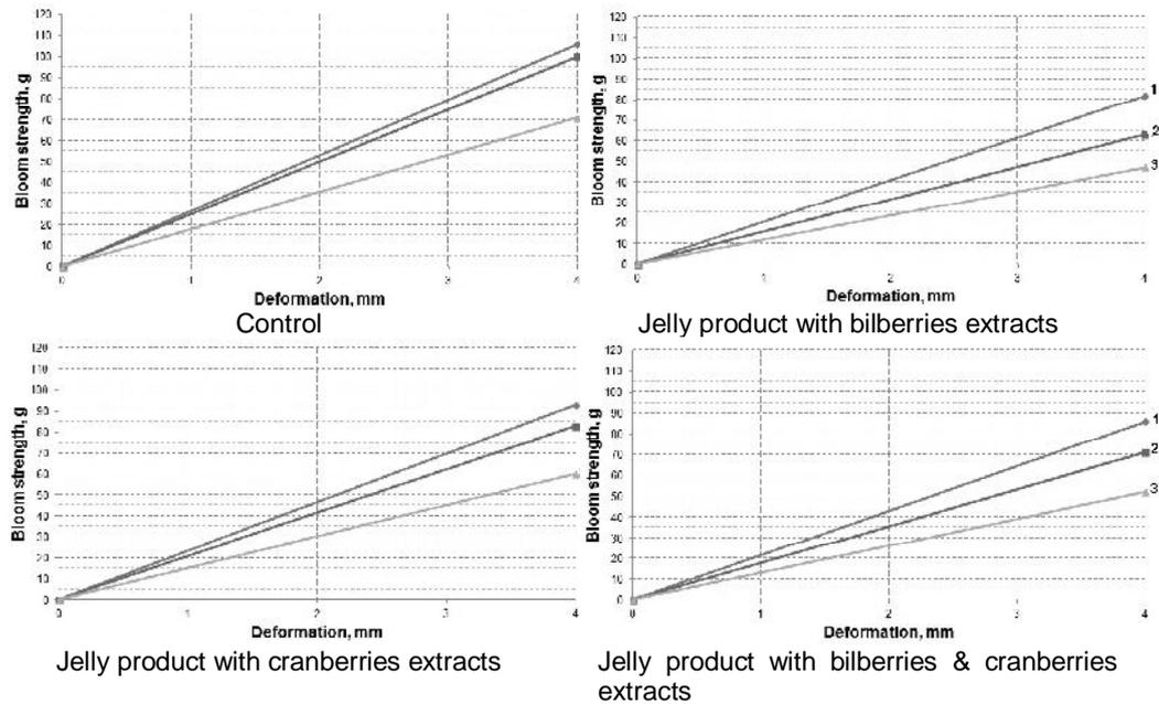
**Figure 5.** Load force change schedules depending on the depth of implementation of Blume indenter for sugar-free jelly products depending on the technology used (by 'ST-2 Structometer'): 1 – traditional; 2 – microwave with gelatin swelling; 3 – microwave without gelatin swelling.
