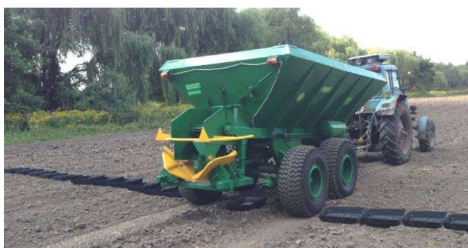
Figure 3. General appearance of the experimental mineral fertiliser top dressing machine with two fertiliser spreading tools, axes of which were set at an angle to horizontal plane, during the field experiment investigations, in which trays were placed along the two directions of spreading.
