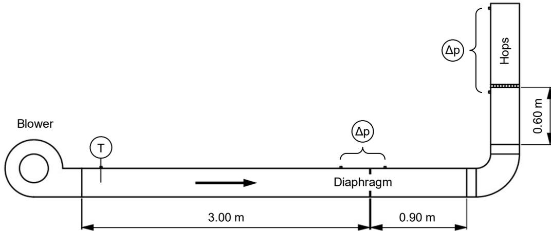
**Figure 1.** Simplified schematic of the test facility.
