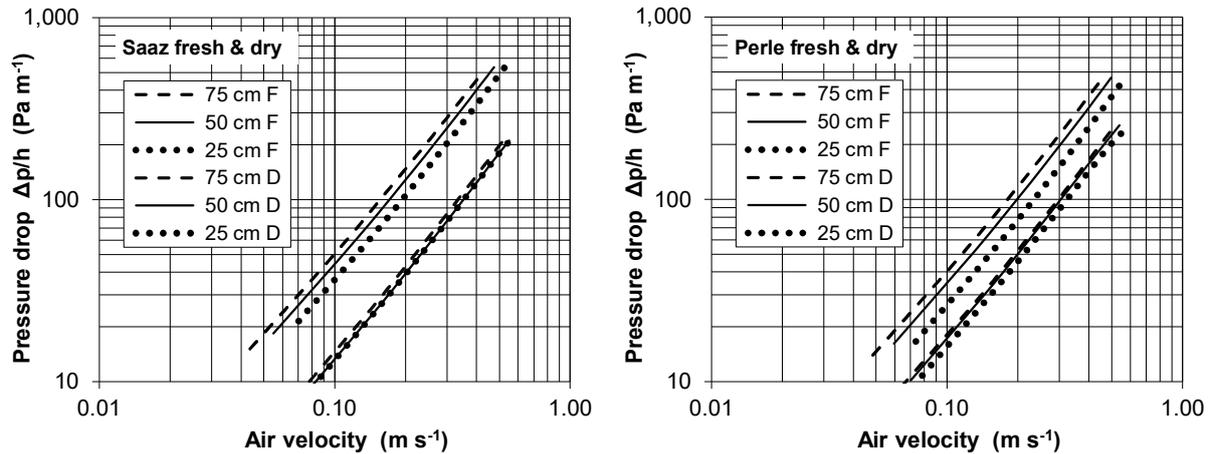
**Figure 4.** Pressure drop of the hop varieties Saaz and Perle, mean values at different air velocities, bed heights, and moisture contents.
