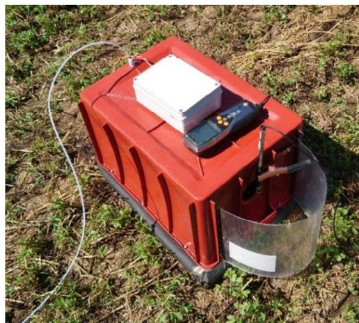
**Figure 1.** Emissions measuring wind tunnel.
