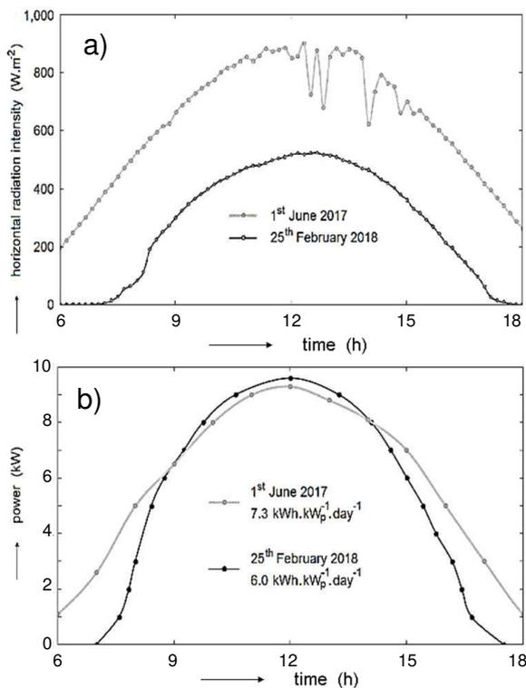
**Figure 4.** Dependence of (a) radiation intensity and b) instantaneous power on the time during two selected sunny days in different seasons.
