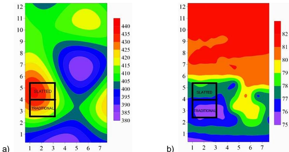
**Figure 7.** Spatial distribution of the average of a) Radiant Thermal Load (RTL) (W m<sup>-2</sup>) and b) Temperature Humidity Index (THI) of the experimental room.
