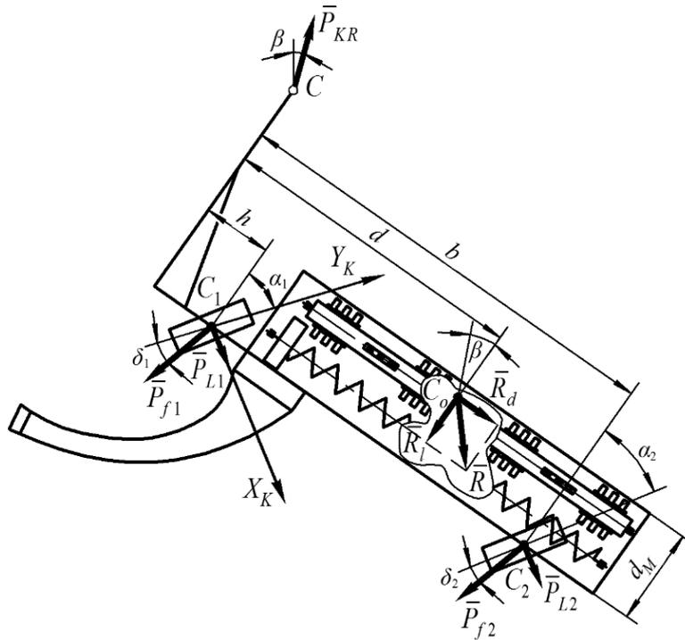
**Figure 3.** Equivalent diagram of an aggregated harvester.
