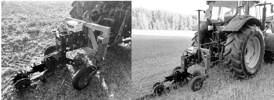
**Figure 1.** Soil scanner iScan+. Left side: soil scanner in 2021, GNSS antenna installed on the scanner. Right side: soil scanner in 2022, GNSS antenna installed in the subframe on top of the pole.
