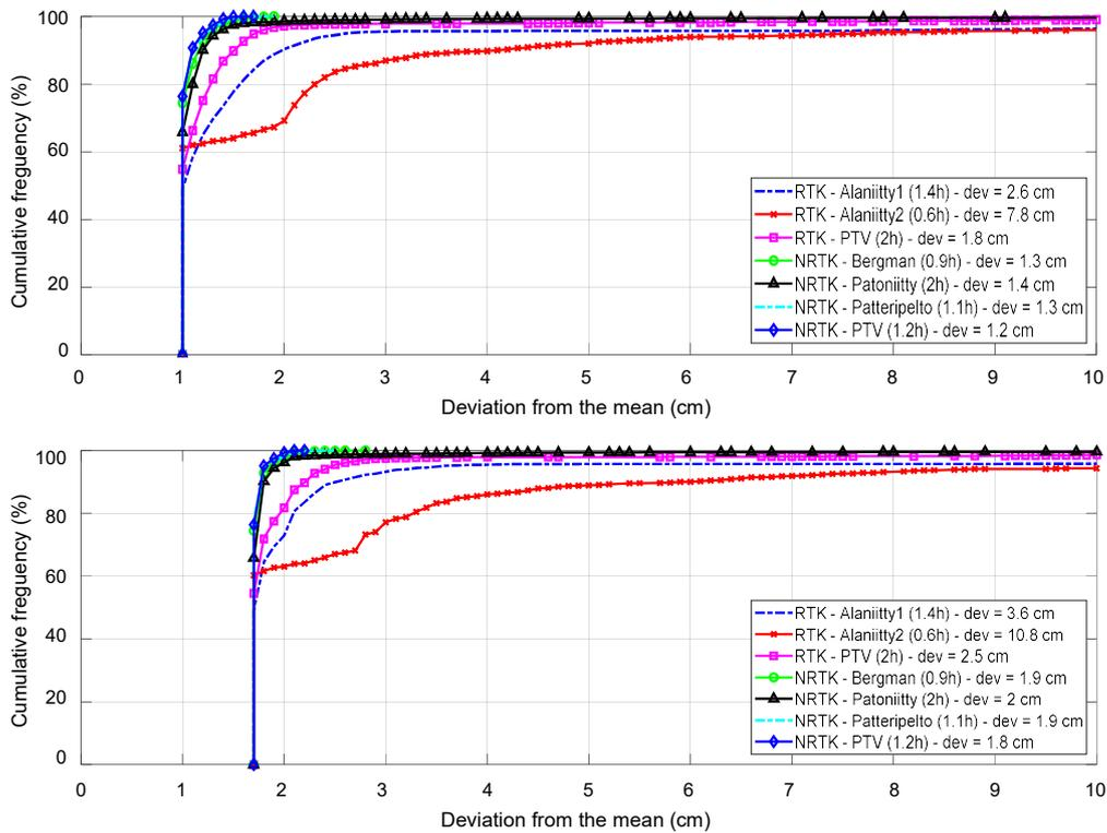
**Figure 6.** Positioning accuracies of the custom RTK and commercial NRTK signals in various fields during soil scanning. Top: horizontal accuracy, bottom: three-dimensional accuracy.
