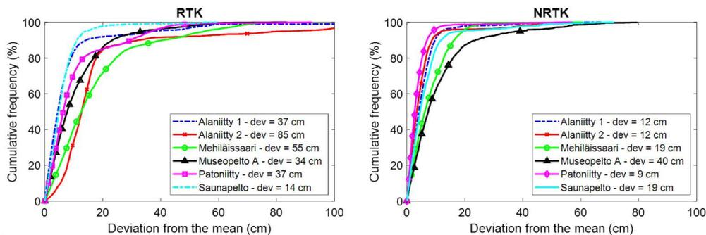
**Figure 7.** Accuracy comparison of the elevation measurement in different fields. Left side: custom RTK. Right side: commercial NRTK.
