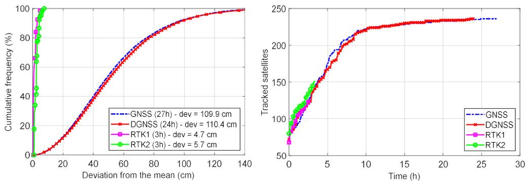
**Figure 5.** Accuracy of the received GNSS and custom RTK-GNSS correction signal in distance. Right side of the figure presents the cumulative number of tracked satellites during recordings.
