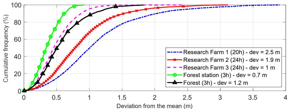
**Figure 4.** Accuracy of the received GNSS signal when recording the base station locations.
