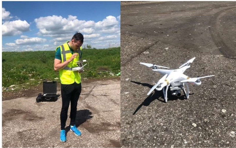
Figure 4. Carrying out a photogrammetric flight with an UAV DJI Phantom 3 Professional.
