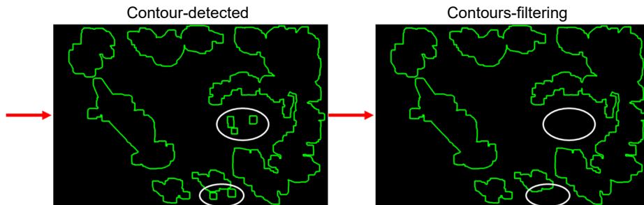
Figure 4. An example of contour-detection and contour-filtering.
