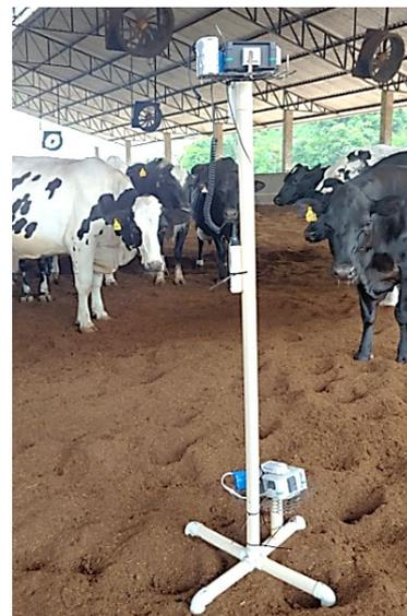
**Figure 3.** Support fabricated for fixing the sensor at a height of 0.25 m.
