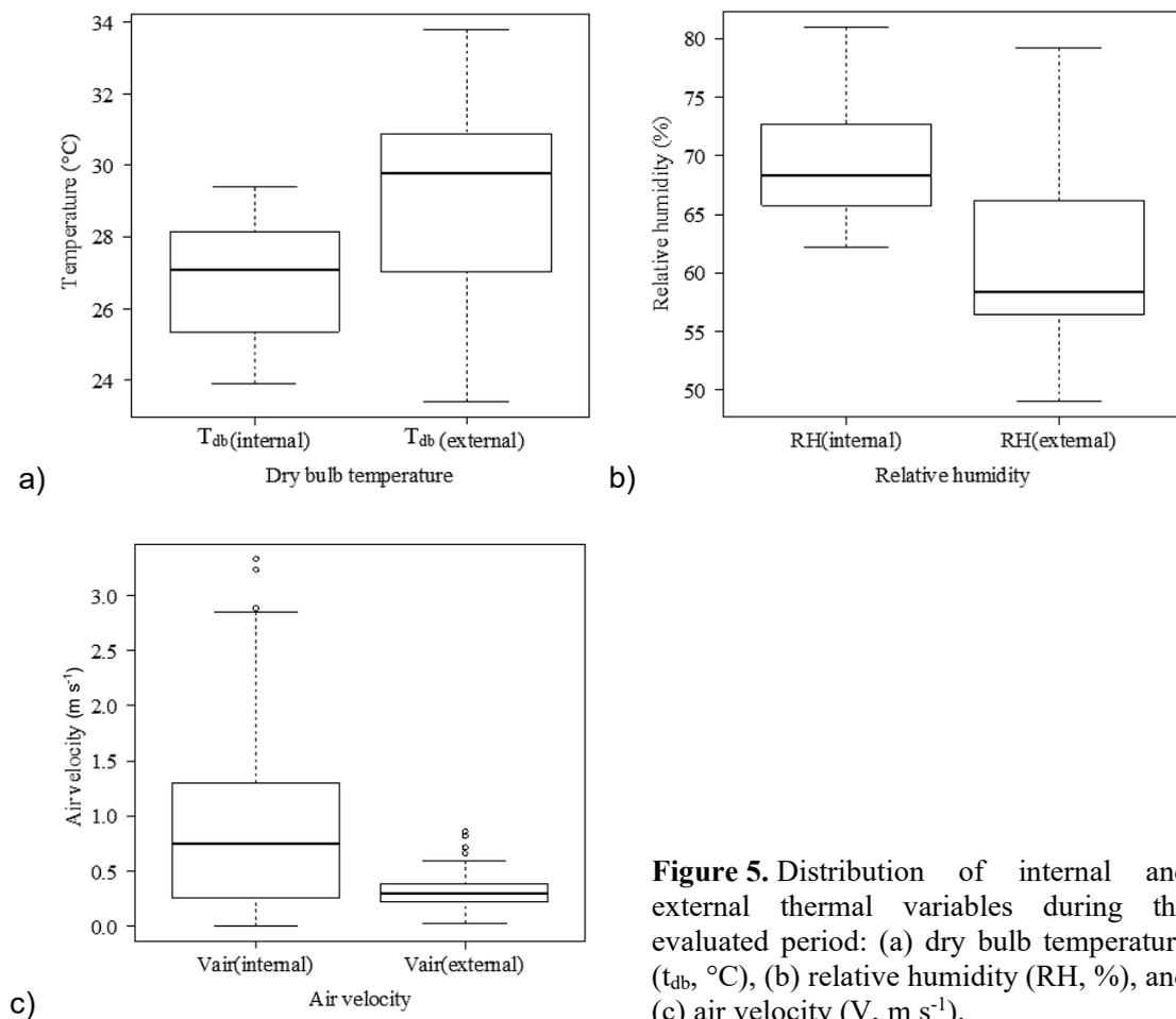
**Figure 5.** Distribution of internal and external thermal variables during the evaluated period: (a) dry bulb temperature ( $t_{db}$ , °C), (b) relative humidity (RH, %), and (c) air velocity ( $V$ ,  $m s^{-1}$ ).
