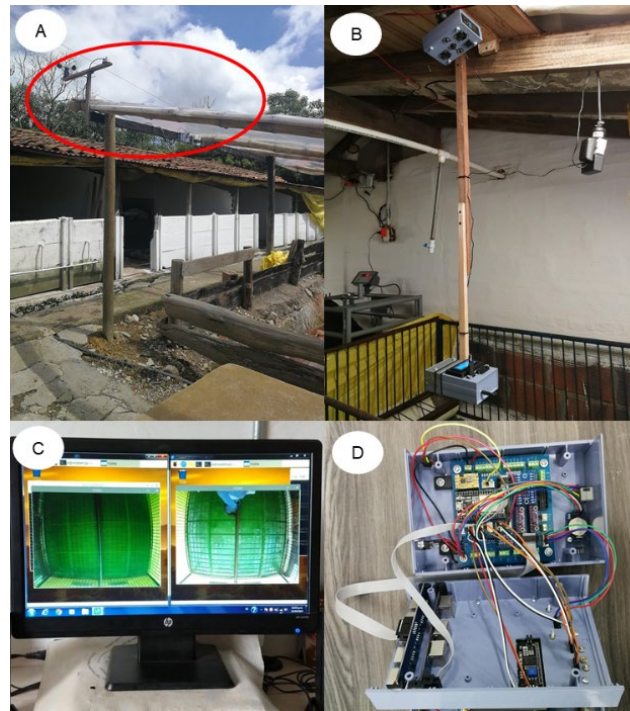
Figure 1. A) External module and experimental piggyery (red circle); B) Internal module location. C) Internal module detail; D) Internal module interior.
