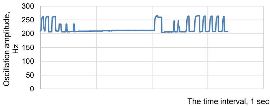
**Figure 18.** Study of resonance frequencies at speed of 10–20 km h<sup>-1</sup>.
