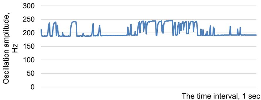
**Figure 19.** Study of resonance frequencies at speed of 40–60 km h<sup>-1</sup>.
