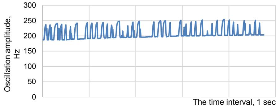
**Figure 20.** Study of resonance frequencies at speed of 80–100 km h<sup>-1</sup>.
