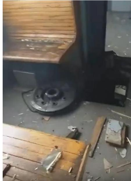
**Figure 1.** Ejection of the flange of the rubber-cord coupling in the passenger compartment.
