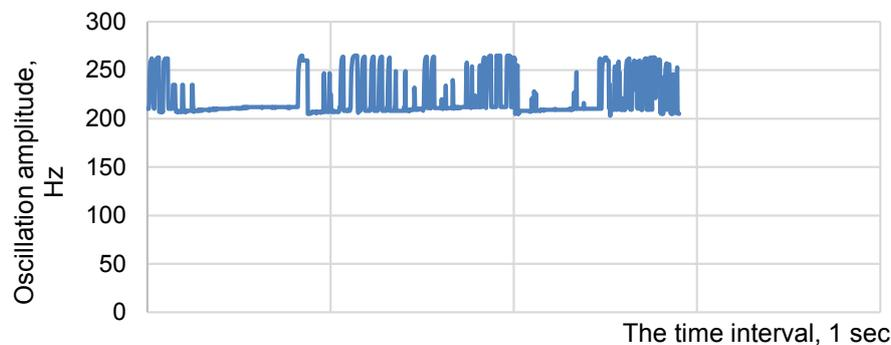
**Figure 21.** Study of resonance frequencies at speed of 110–120 km h<sup>-1</sup>.
