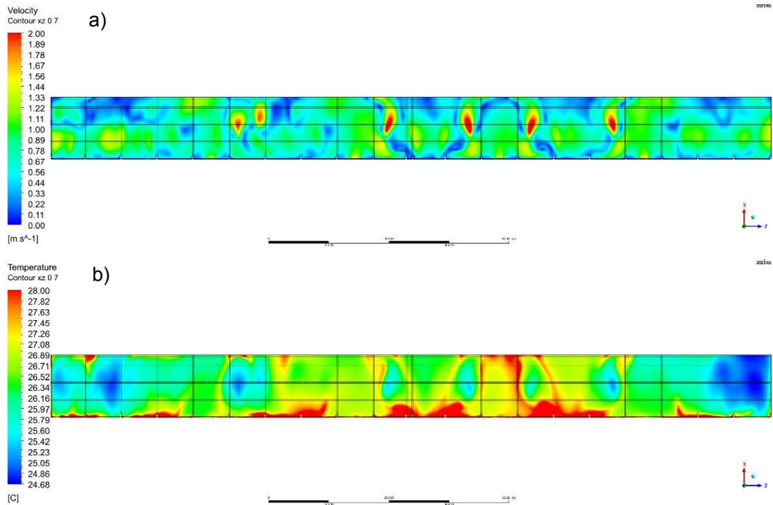
**Figure 4.** Velocity field,  $\text{m}\cdot\text{s}^{-1}$  (a), and temperature field,  $^{\circ}\text{C}$  (b), in the poultry house along the  $zx$  axis at a height of 0.7 m from the floor level.
