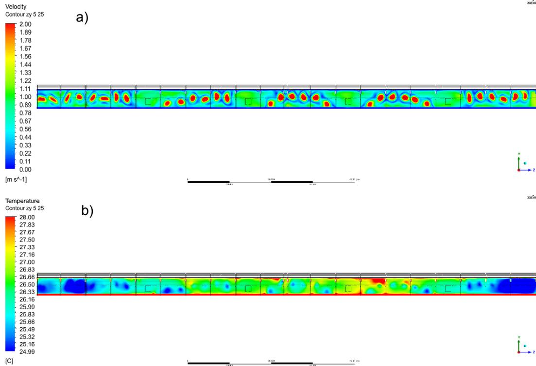
**Figure 6.** Velocity field,  $\text{m s}^{-1}$  (a), and temperature field,  $^{\circ}\text{C}$  (b), in the poultry house along the  $zy$  axis at 5.25 m from the side wall.
