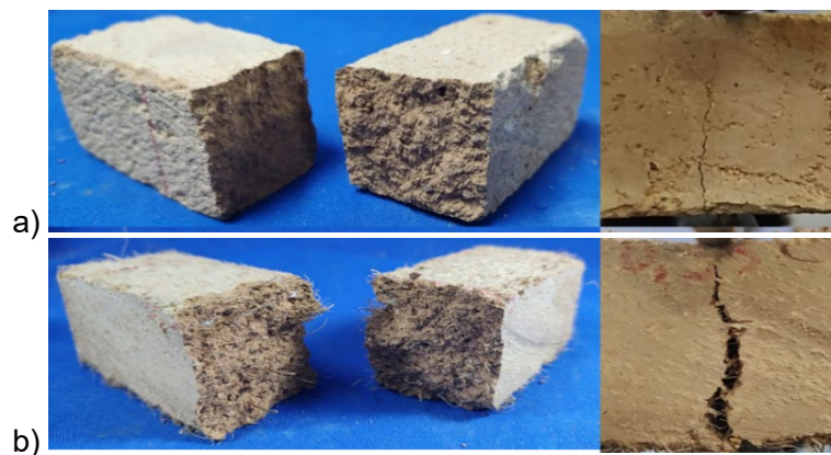
Figure 9. Adobe samples after the bending test:(a) Reference and (b) 2% fiber.
